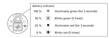
\* When the battery charge is low, first the front derailleur will stop operating, and then the rear derailleur will stop operating. When the battery is fully spent, the derailleurs will stop at the positions where they were last shifted to. If the battery indicator is illuminated red, it is recommended that you recharge the battery as soon as possible.
